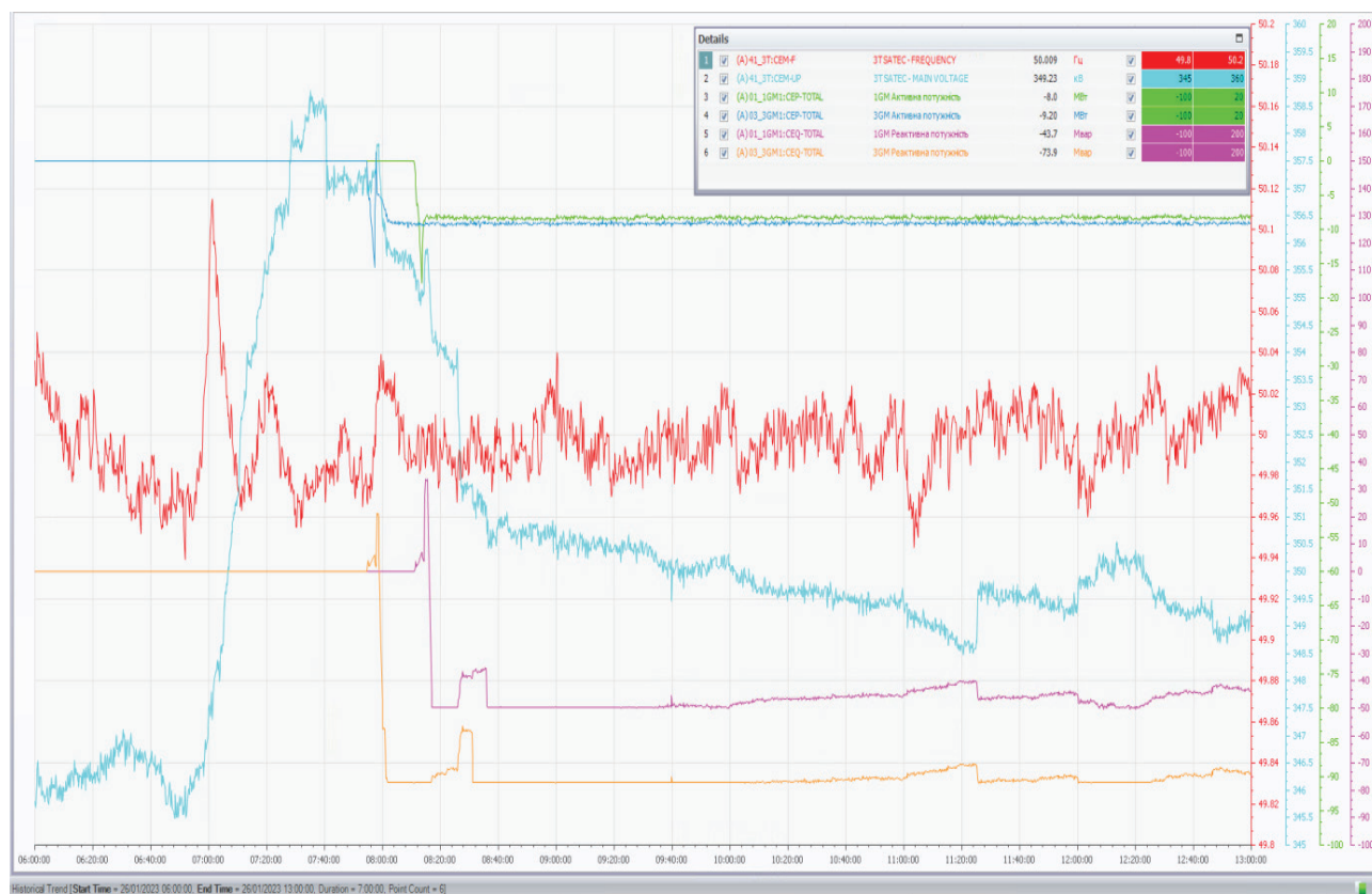
Figure 2. The transient was registered at the Tashlyk pumped storage power plant (TPSPP) after a missile attack on the power system of Ukraine on January 26, 2023.
