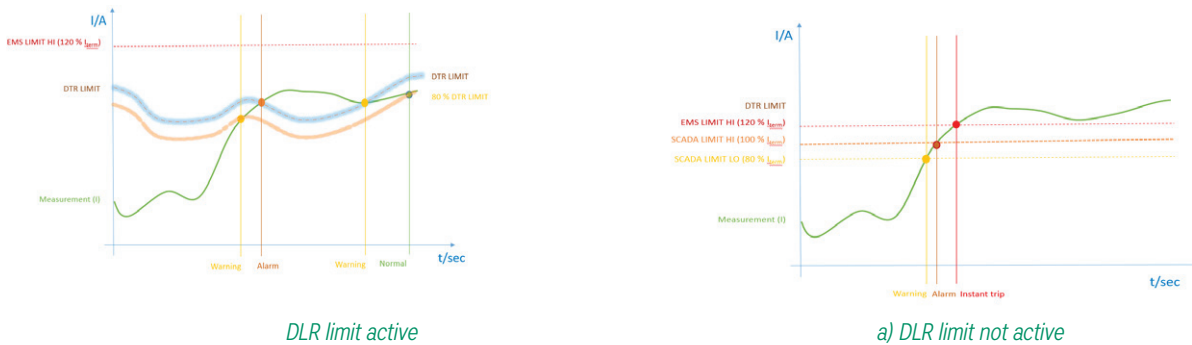
Figure 8. Example of activation of limits on real time data with static limits and DLR limits active
