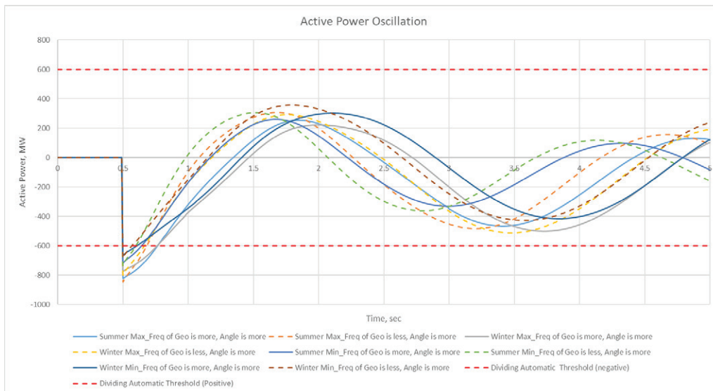
Figure 4. Active power swing at interconnector in case \Delta\delta = 40^\circ , when phase angle of Georgian power system leads the one of neighboring power system in a moment of synchronization
