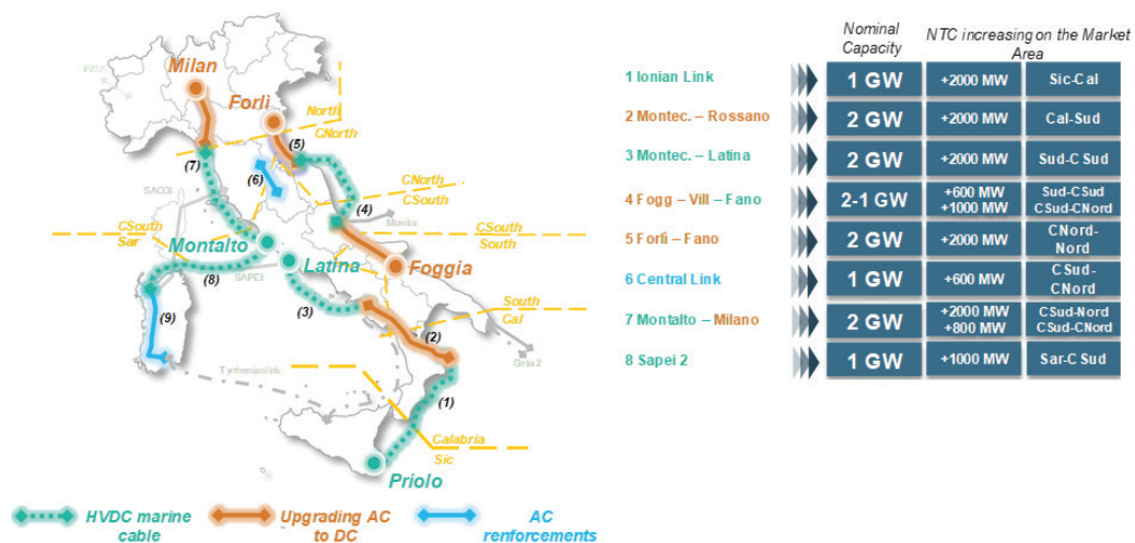
Figure 1. Overview of the entire Hypergrid project and associated NTC (Net Transfer Capacity)
