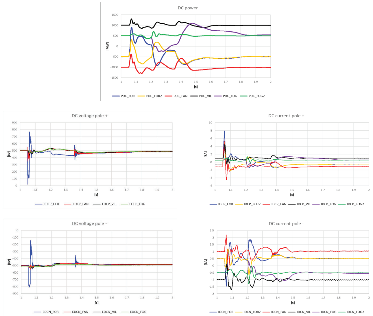
Figure 11. Case id.C2 with HVDC breakers. DC power (top), voltage (middle) and current (bottom)
