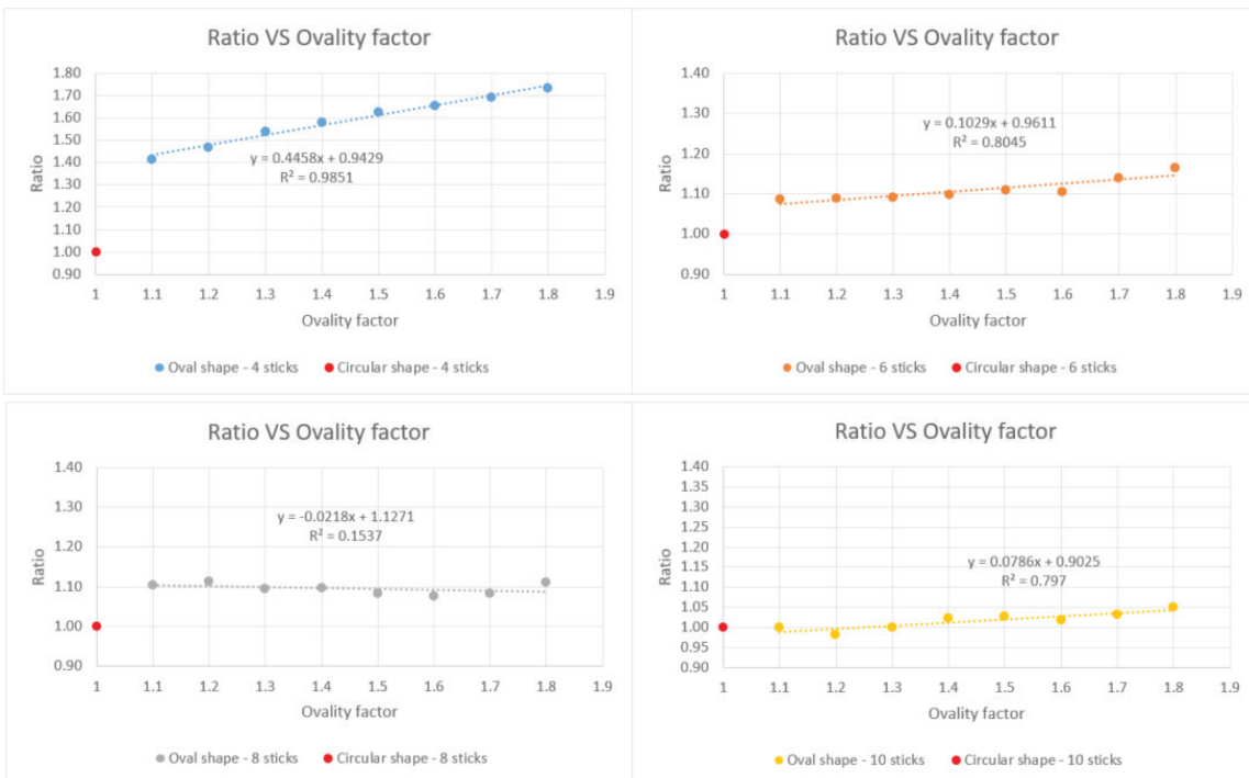
Figure 9: Ratio VS ovality factor for different number of duct sticks (Stress analysis)
