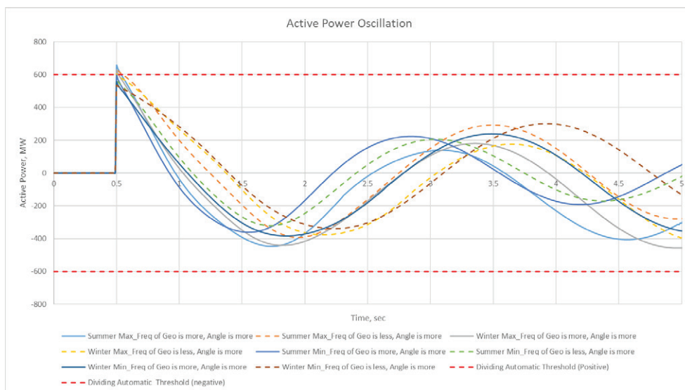
Figure 7. Active power swing at interconnector in case \Delta\delta = 30^\circ , when phase angle of Georgian power system lags the one of neighboring power system in a moment of synchronization
