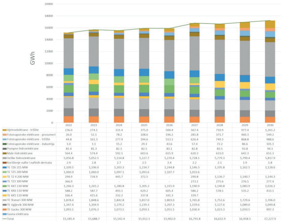
Figure 24. Trajectories of the amount of electricity produced by type of plant in B&H 2022-2030 [2]
