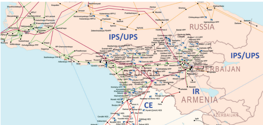
Figure 8. Synchronous zones around GE
