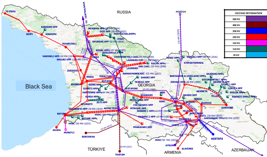
Figure 12. Existing and planned Georgian transmission system 2023-2033
