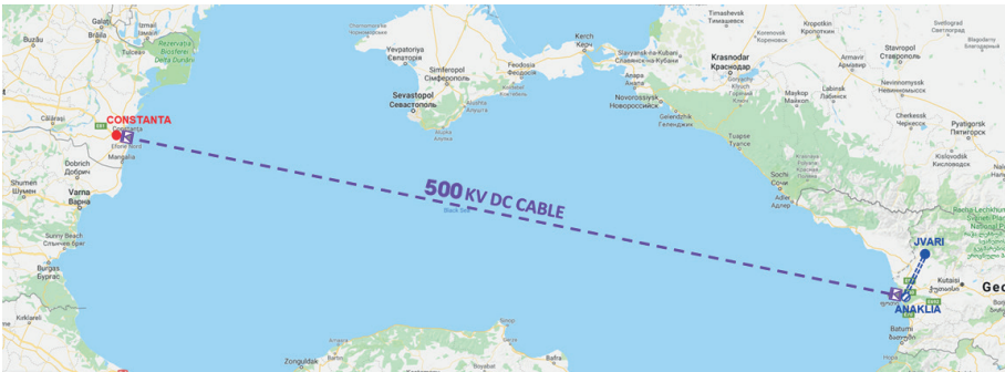
Figure 13. GE-RO Black Sea submarine cable
