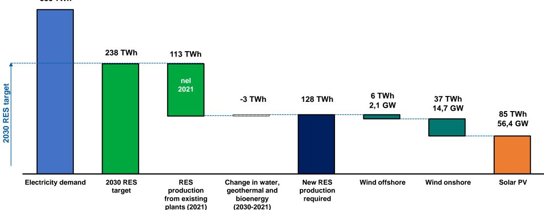
To reach the decarbonisation targets of the new National Energy and Climate Plan (NECP), in Italy it will be necessary to double the total renewable production and quadruple the photovoltaic one. The geographical location of such significant volumes must also be addressed through ad-hoc policy measures.
